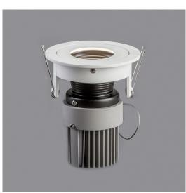
The product is made of aluminium alloy through die-casting, shaped by CNC machine, then treated by podwer coating. LED driver is installed externally. COB LED or LED QR-CB51 or QR-CB51 light source is used, the radiation angle is nonadjustable. 50,000 hours lamp life at 50°C
