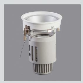
The lighting body is made of aluminium alloy through die-casting, shaped by CNC machine, then treated by power coating. Reflector is made of special alloy through die-casting and treated by special technics, heat-resistant and anti glare. Fixed fitting.
