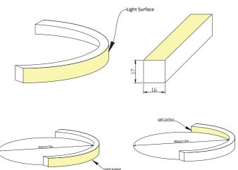
The Flex Tube is an outdoor rated flexible LED tube. It features a bend diameter of 300mm and it can be cut to length every 83.3mm. It features an IP68 submersible rating, suitable for any exterior applications. It is sold on a spool of 10m and it is controlled via DMX-SPI.
